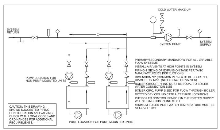
Figure 9. Hydronic Piping - Primary-Secondary, Reverse-Return.
